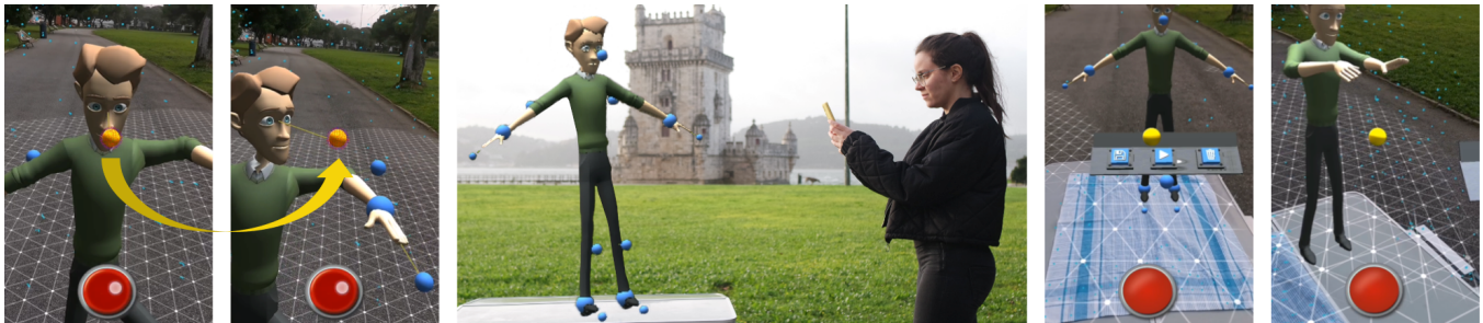
Figure 1: With AR-Pose a smartphone functions as a 3D cursor (yellow sphere) that selects and manipulates IK handles (blue spheres) for articulating the underlying rig of a humanoid character. Through a control panel placed in the workplace, a user can then define and save a sequence of poses to latter reproduce them as an animation.
